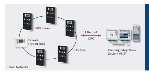
The 5000 Series can be connected by means of the CAN-Bus and can be integrated into the Building Integration System
